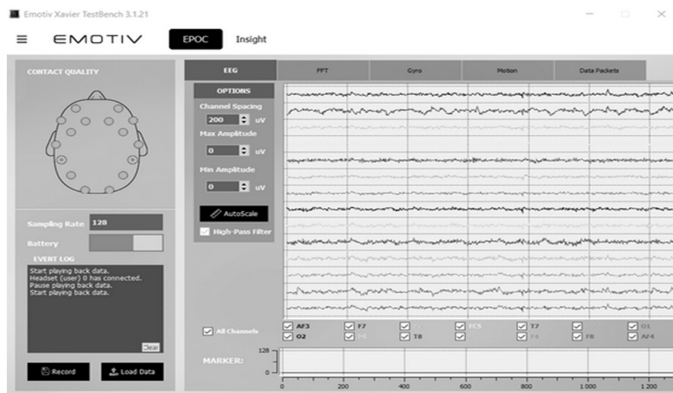
Figure 4. Emotiv EEG Testbench© interface that shows the progress of the raw EEG data being collected wirelessly from the Emotiv's 14 electrode sensors.
