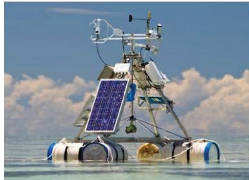
Figure 2. Pontoon mounted Eddy Covariance unit at Heron Reef
