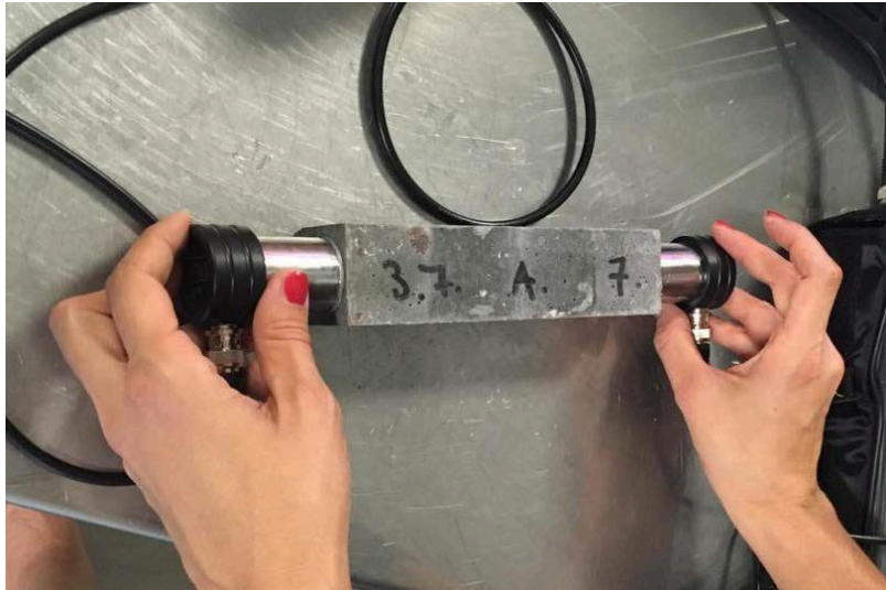
Figure 17 - The right position of tested sample during ultrasonic test
