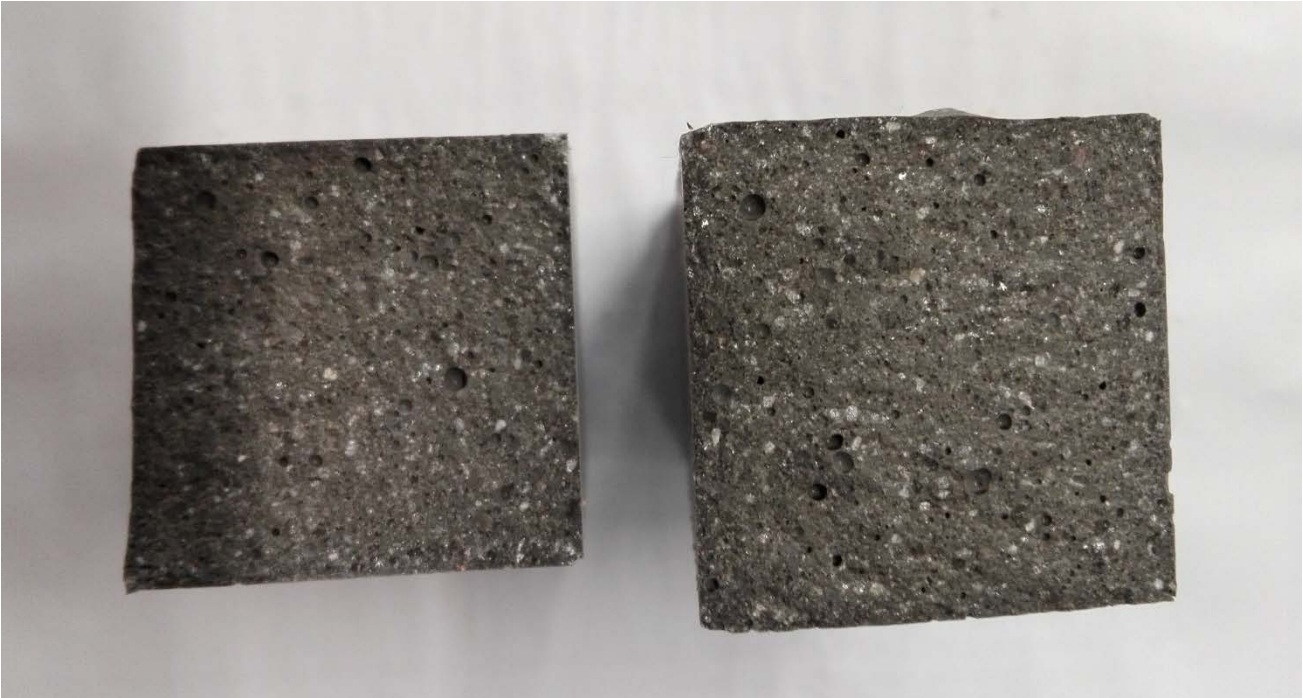
Figure 26 - Sample A after tensile bending strength test – 100 cycles
