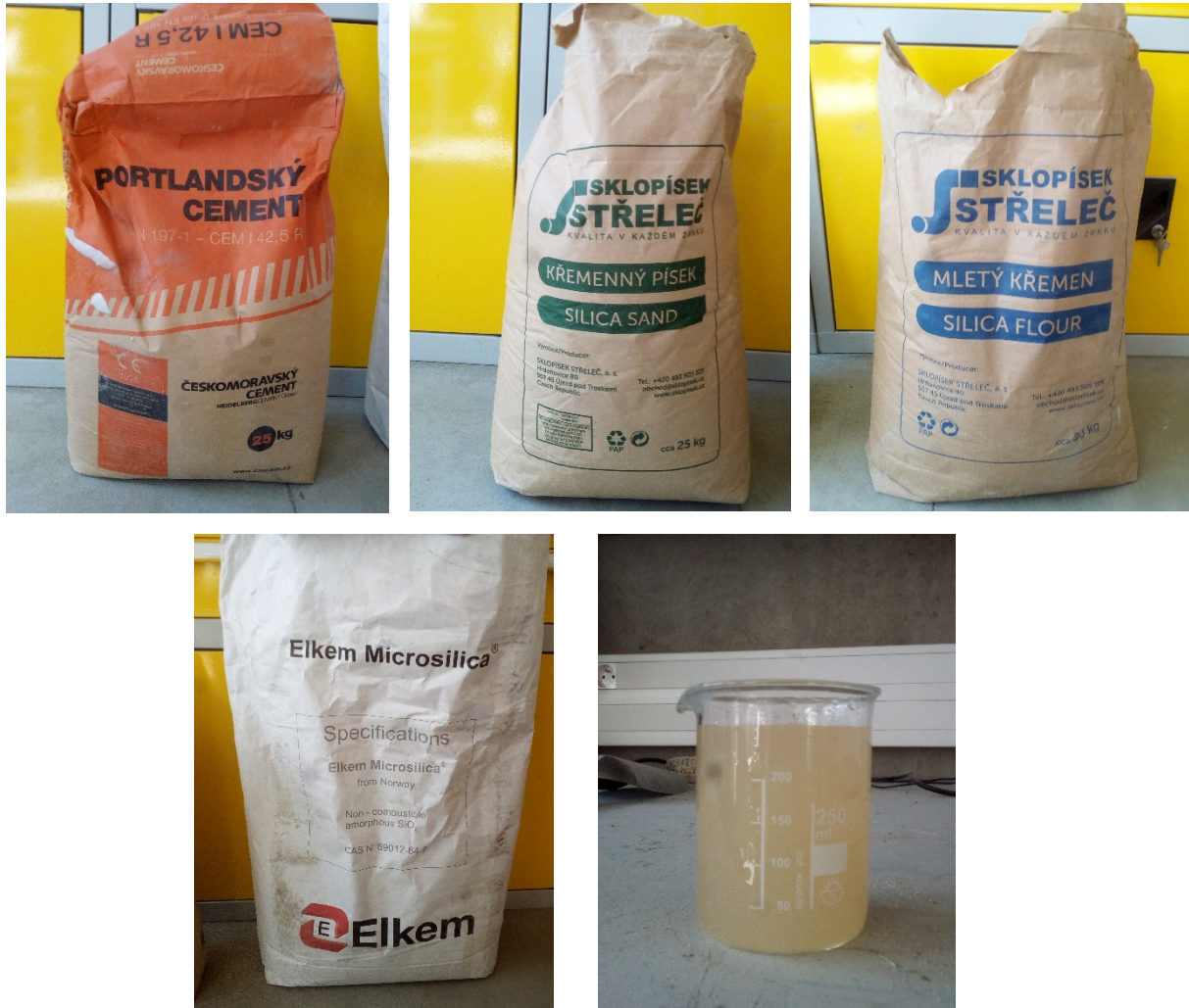
Figure 9- Materials used for preparation of HPC (cement, silica sand, silica flour, silica fume, superplasticizers)
