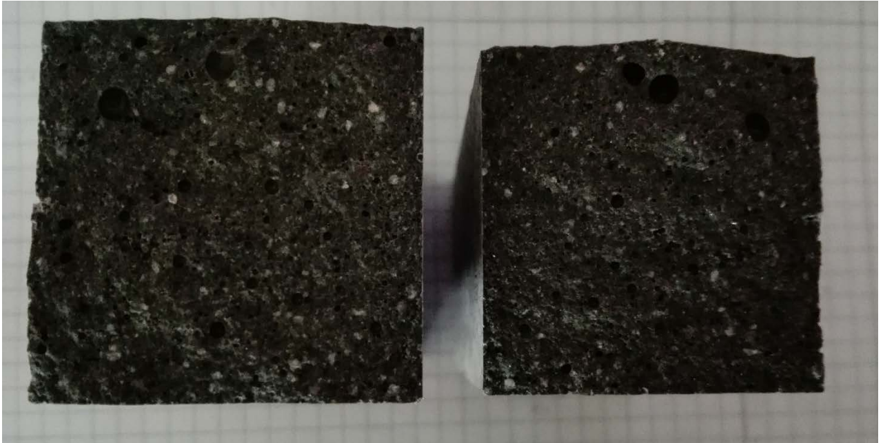
Figure 25 - Sample C after tensile bending strength test – 75 cycles
