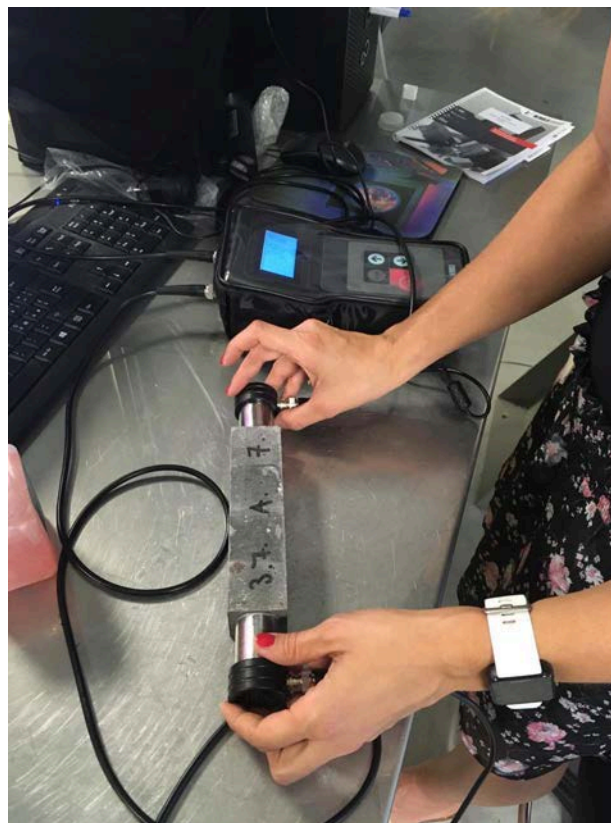
Figure 10 - Measuring of the pulse speed using ultrasonic pulse method
