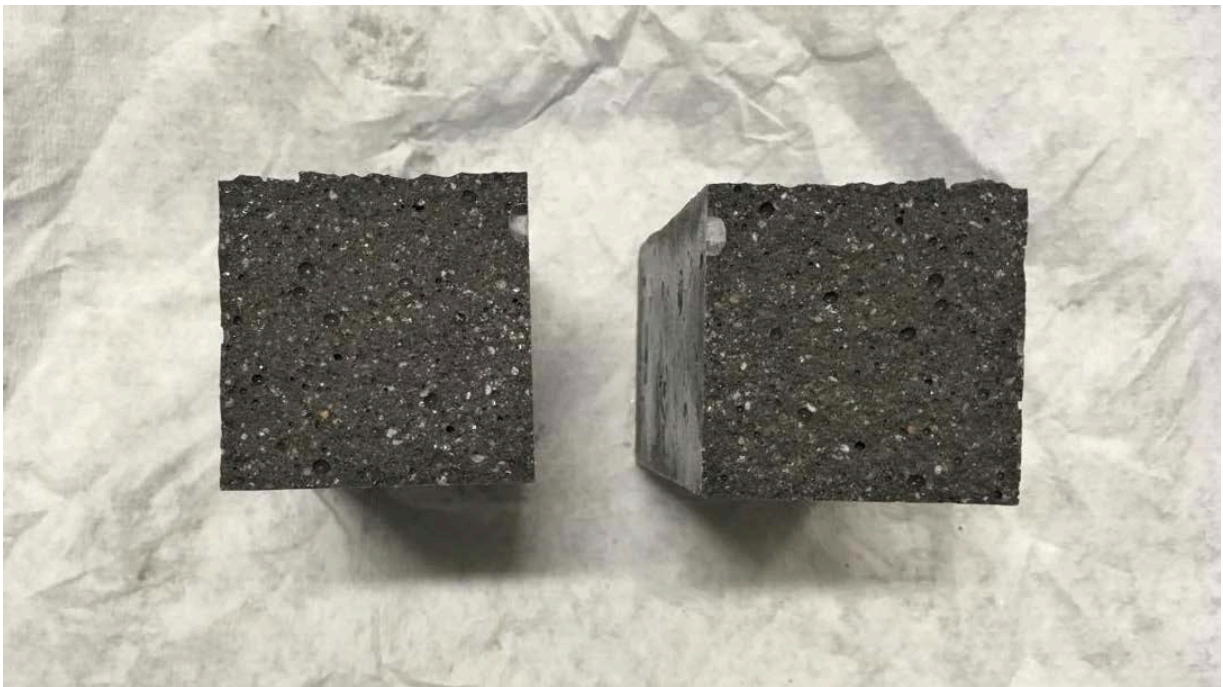
Figure 21 - Sample B after tensile bending strength test – 50 cycles
