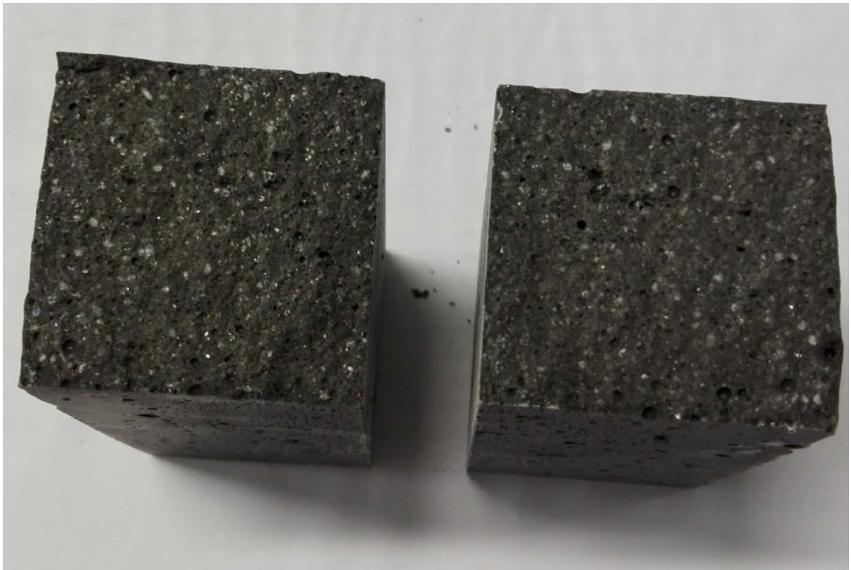
Figure 28 - Sample C after tensile bending strength test – 100 cycles
