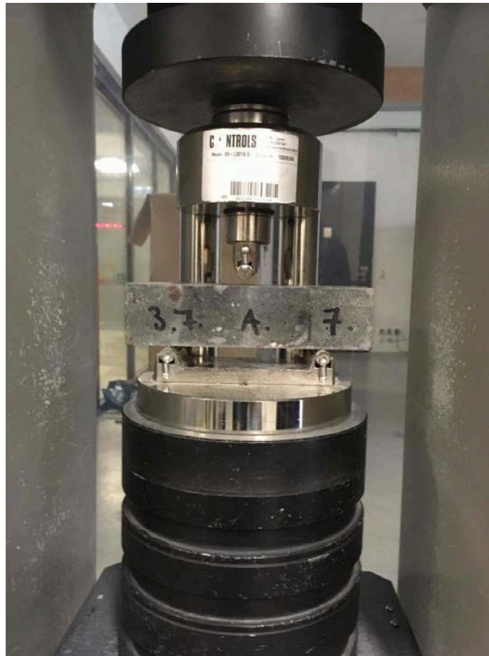
Figure 18 - The right position of tested sample during testing tensile bending strength
