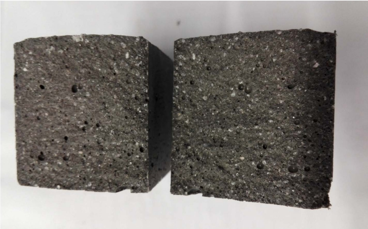
Figure 27 - Sample B after tensile bending strength test – 100 cycles
