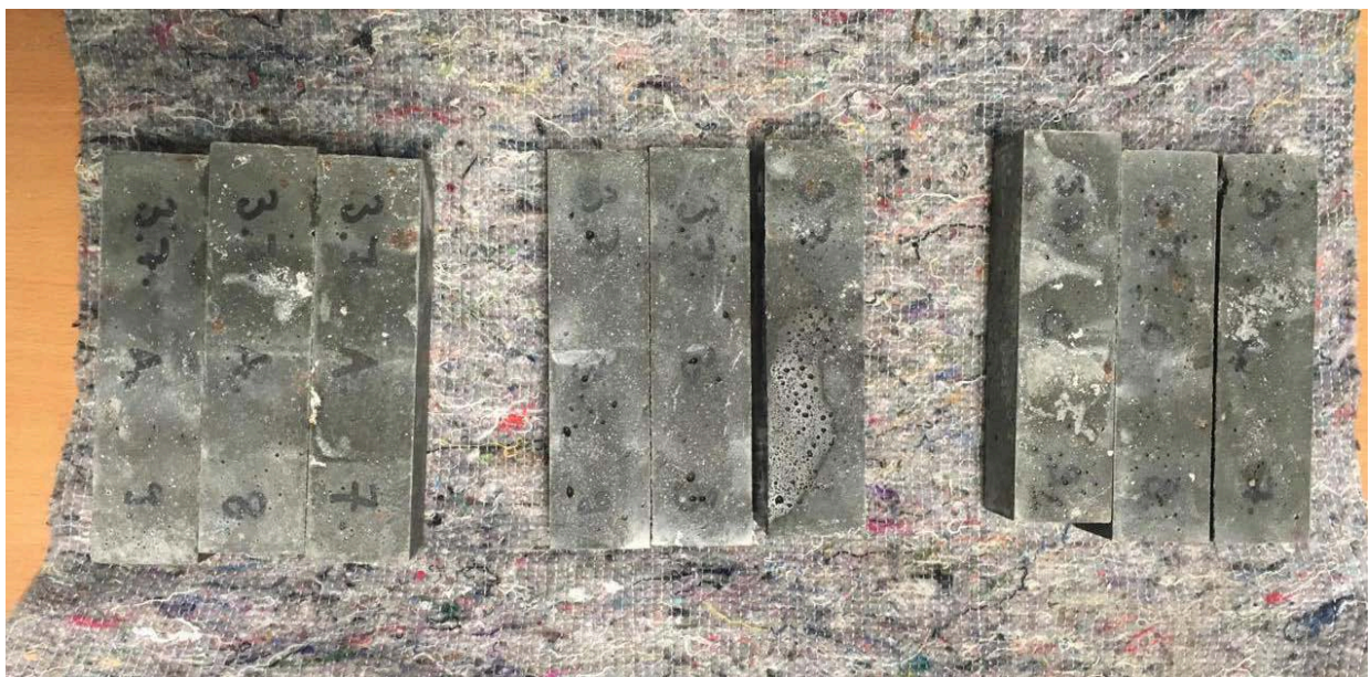
Figure 19 - The samples after freeze-thaw resistance test
