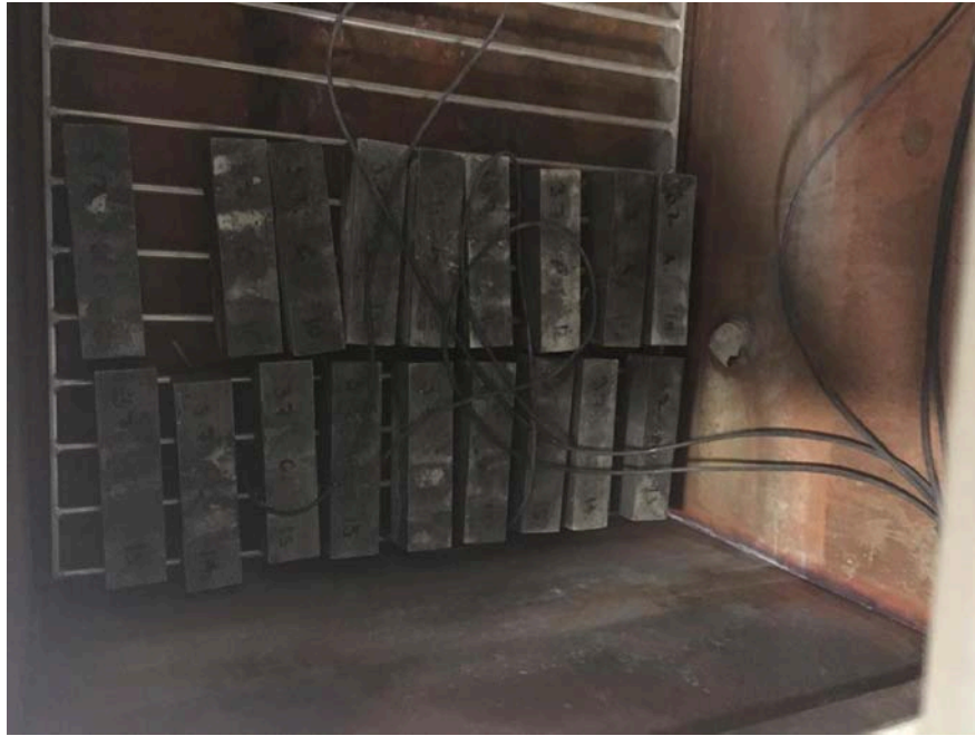
Figure 16 - Samples in the freezer during the freeze-thaw resistance test
