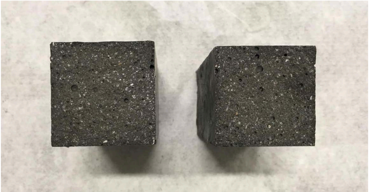
Figure 20– Sample A after tensile bending strength test – 50 cycles
