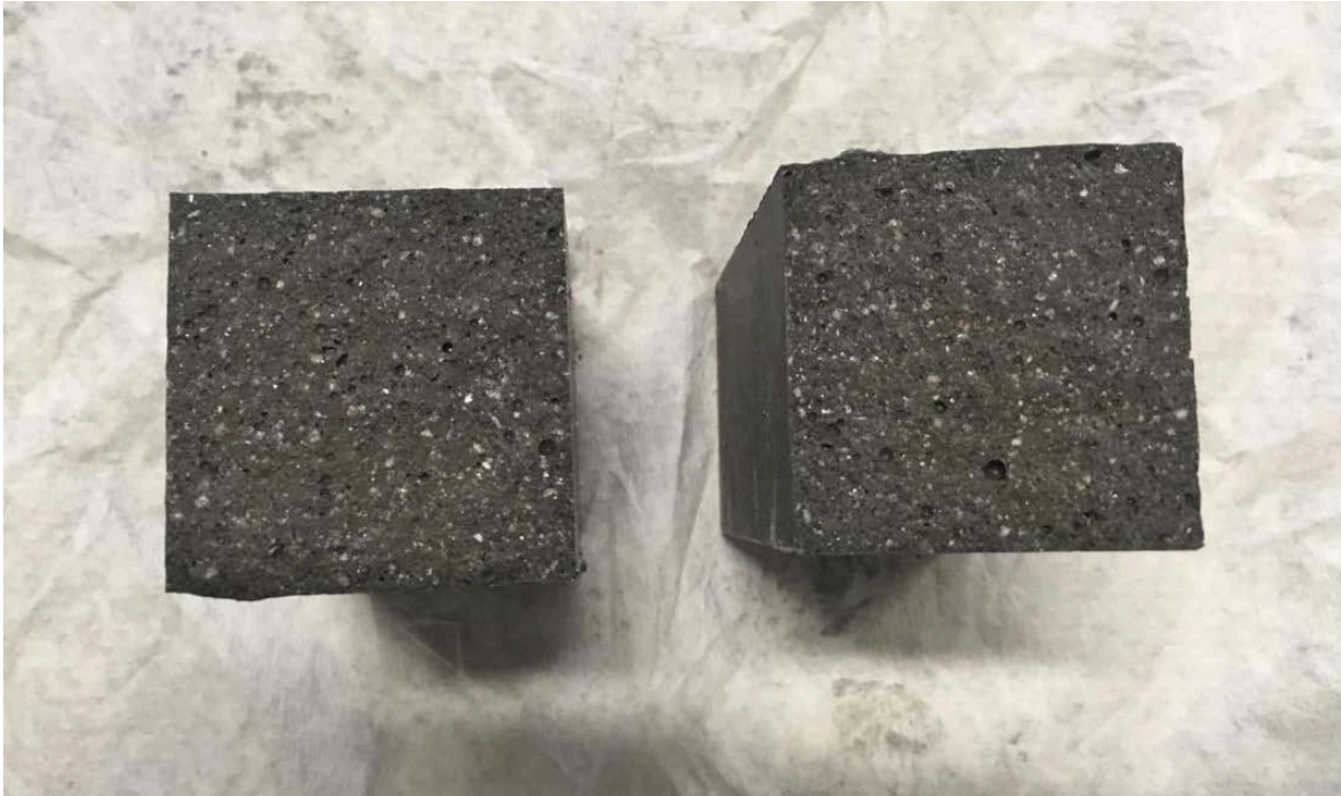
Figure 22 - Sample C after tensile bending strength test – 50 cycles
