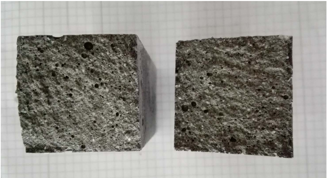
Figure 24 - Sample B after tensile bending strength test – 75 cycles
