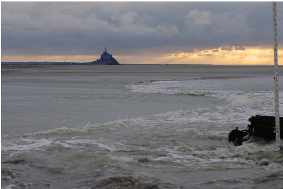
(D) Tidal bore about 5 s after it reached the ADV unit (Photograph H. CHANSON) - Note the curve shape of the bore front and, in the background, the dark colour of the bore front advancing on the sand banks
