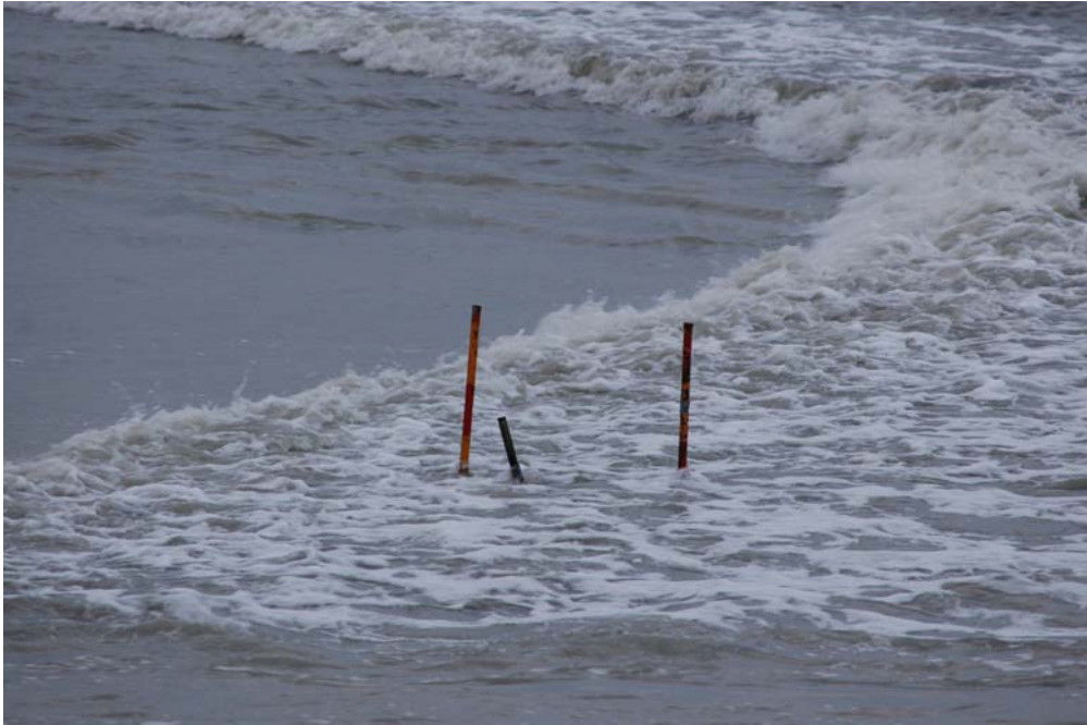
(C) Details of the tidal bore roller, shortly after passing the ADV unit (Photograph D. MOUAZE) - Note the transverse curvature of the bore front
