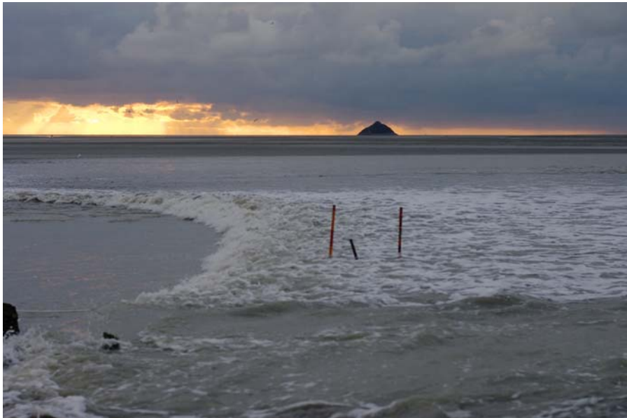
(I) Tidal bore about 2 s after it reached the ADV unit (Photograph H. CHANSON)
