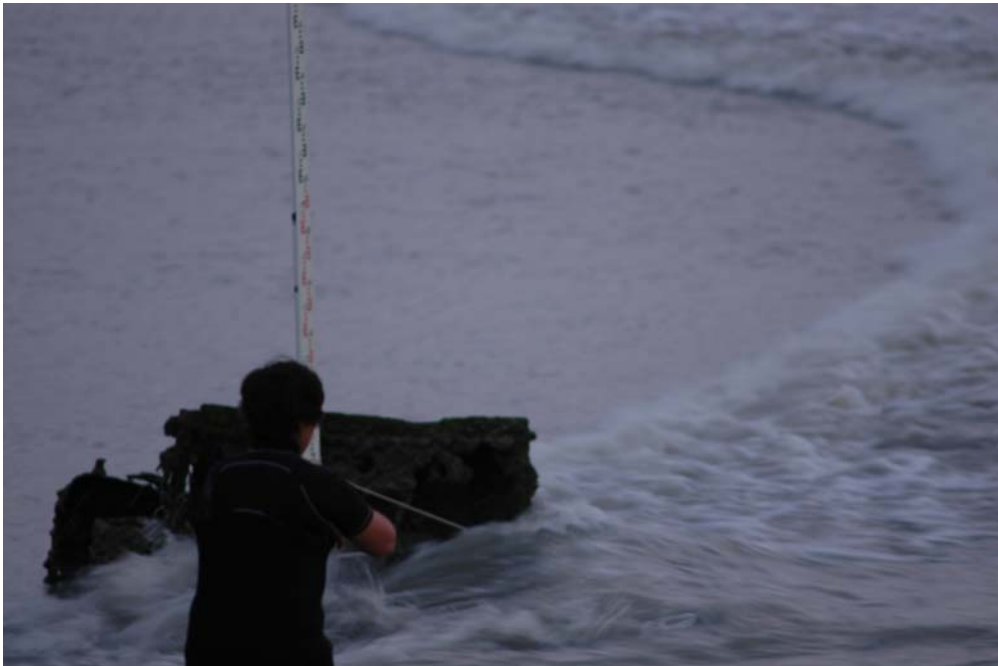
(B) Tidal bore passing the WWII German truck with Frederique LARRARTE, in the foreground, timing the tidal bore celerity (Photograph D. MOUAZE) - The ADV unit was behind the WWII German truck
