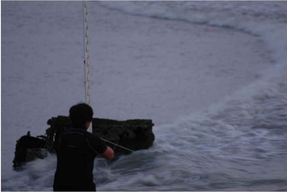
(E) Tidal bore passing the WWII German truck with Frédérique LARRARTE, in the foreground, timing the tidal bore celerity (Photograph D. MOUAZE)
