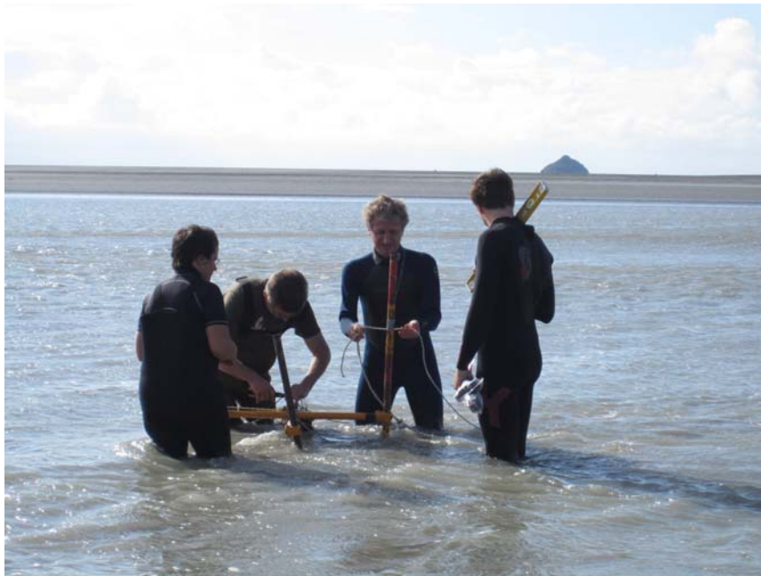
(A) Tripod supporting the ADV system on 24 Sept. 2010 at 16:40 (Photograph F. MURZYN) - From left to right, Frederique LARRARTE, Dominique MOUAZE, Hubert CHANSON and Bruno SIMON - Dominique MOUAZE was preparing the ADV unit with its head pointed towards him
