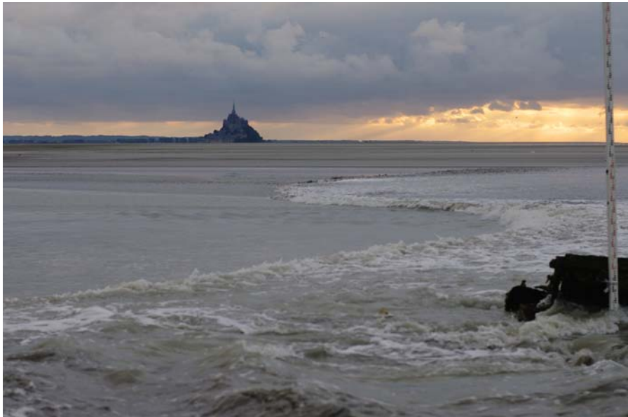
(K) Tidal bore about 5 s after it reached the ADV unit (Photograph H. CHANSON) - Note the curve shape of the bore front and, in the background, the dark colour of the bore front advancing on the sand banks
