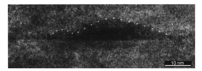
FIG. 1. A  $\langle 110 \rangle$  cross-section HREM image of buried In<sub>0.6</sub>Ga<sub>0.4</sub>As quantum dots showing two lens-shaped dots partially overlapped. The boundaries are highlighted using white stars.
