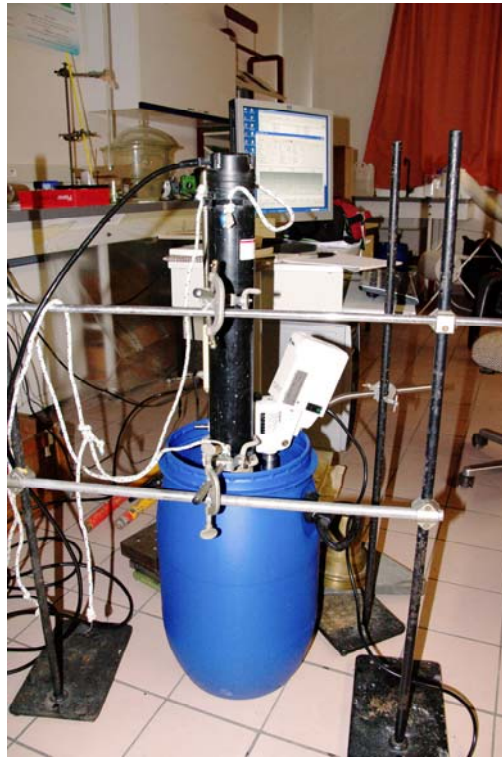
(A) SSC = 0 g/l (no added sediment) - The ADV system is in the middle with two water mixers on each side behind
