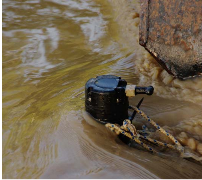
(A) Murky flood flow past the ADV - Flood flow direction from left to right
