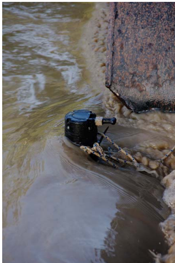
(D) Details of the ADV - On 10 Sept. 2010 at 19:05 about 50 minutes after the tidal bore - Flow velocity from left to right - Note the dark brown colour of the waters highlighting the large suspended sediment load
