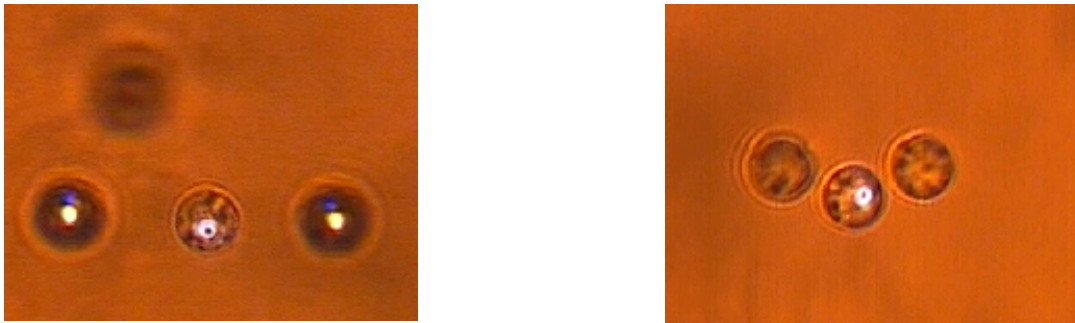
Figure 4. Optical images of polystyrene beads trapped in the three beams before (left) and after (right) Z steering of the dual trap.
