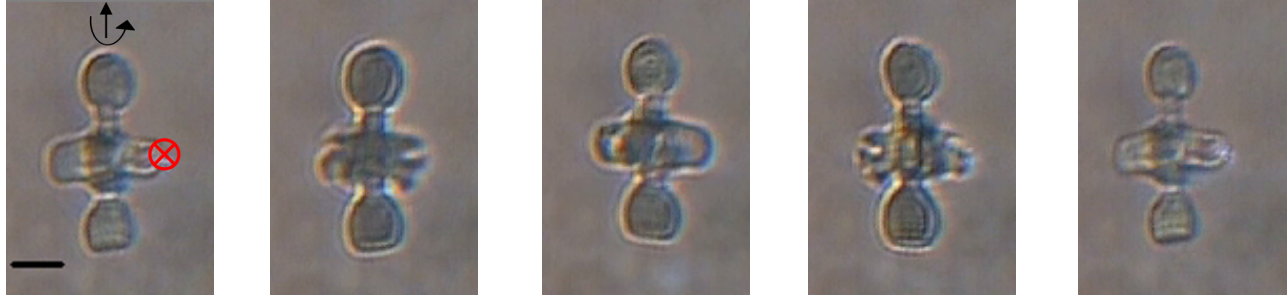
Figure 6. A sequence of bright field microscope images of the rotating paddle-wheel. The frames are 14 ms apart, giving a rotation rate of 2 Hz. In the first frame the position and direction of propagation of the “pushing beam” is indicated by the marker on the paddle. The scale bar is 3 \mu\text{m} .
