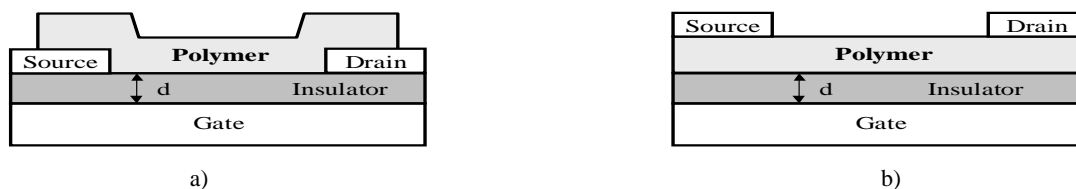
Figure 1: Typical test TFT structures for PFETs: a) Bottom contact configuration; b) Top contact configuration
