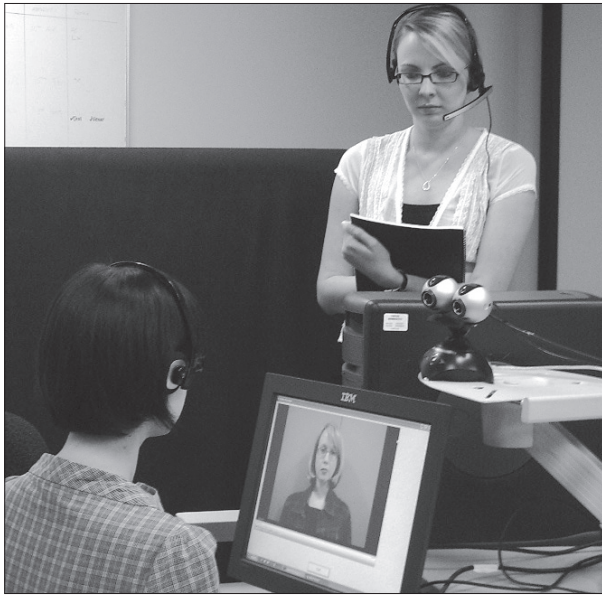
Fig. 1. Participant seated in front of telerehabilitation system, with a demonstration video being screened to the participant while the face-to-face speech–language pathologist observes the participant from the far side of the monitor.
