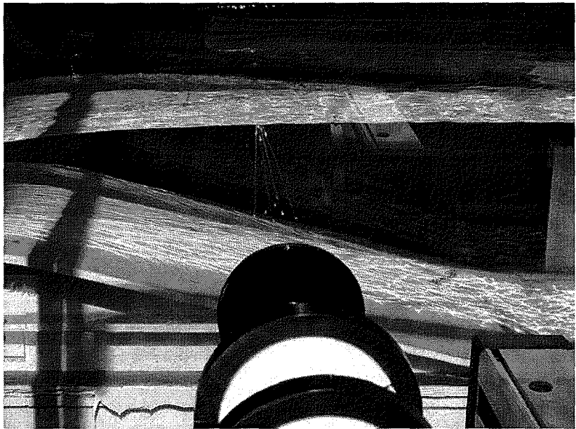
Figure 12. LDV measurements in hydraulic jumps at the University of Caen (France) in 2002. Flow from right to left. The hydraulic jump is formed by a round-shaped obstacle situated on the bottom of the channel. The four Laser beams (two green and two blue) converge at the measurement point. With this 2D system, both horizontal and vertical components of the velocity are simultaneously recorded.
