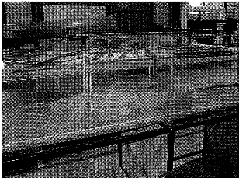
Figure 13. Hydraulic jump at the University of Queensland, flow from left to right, d_1 = 0.018 m, x_1 = 0.75 m, Fr = 5 , Re = 37800 , U_1 = 2.1 m/s, PD inflow conditions. Photo by Hubert Chanson.
