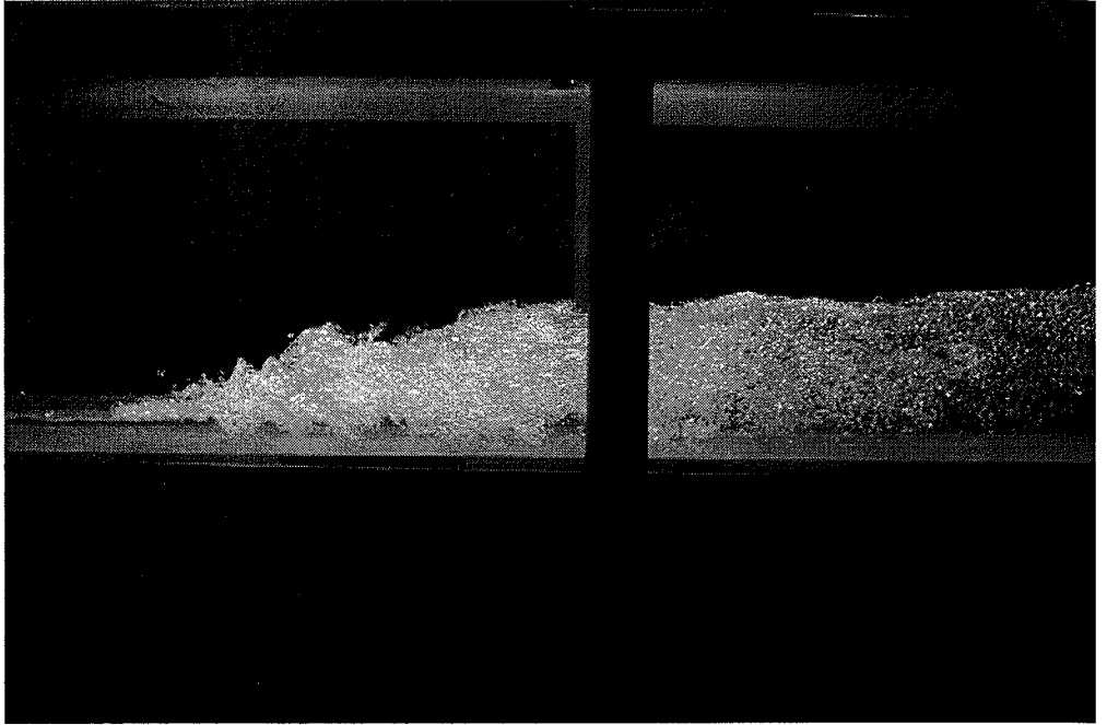
Figure 3. Hydraulic jump during laboratory experiments at the University of Southampton (School of Engineering and the Environment, Southampton, UK), Flow from left to right, Fr = 3.65 , d_1 = 0.032 m. Photo by Frédéric Murzyn.
