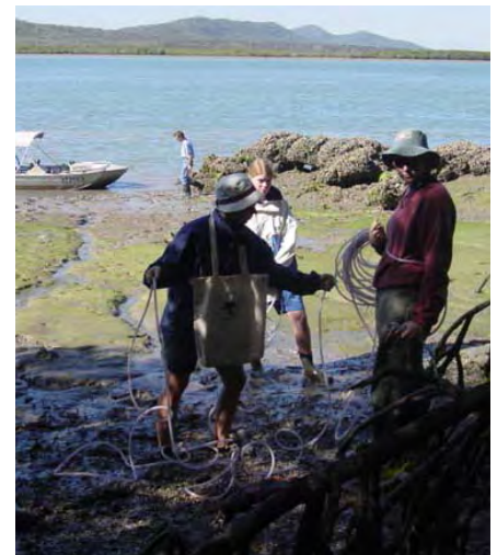
Figure 46. U-tube and ruler used for elevation readings where dense vegetation restricted usage of dumpy level and staff.
