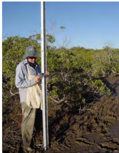
Figure 45. Field survey: staff viewed with dumpy level.
