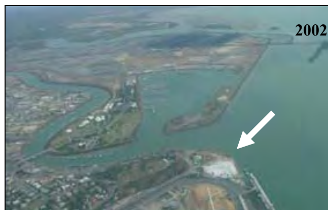
Figure 25(a) & (b). Oblique aerial photos showing the advancing developments in Auckland Inlet. The white arrow denotes the same point in both years. In 1947, the Shell Terminal is visible on reclaimed land, Auckland Point. In 2002, there has been further reclamation, construction and modification, particularly opposite Auckland Hill, where the ‘new’ harbour and port developments may be seen. (Source: (a) Gladstone Port Authority; (b) Norm Duke).
