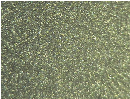
FIGURE 5: Optical microscope image of screen printed Ag electrode ( \times 600 ) by using Ag paste (1).
