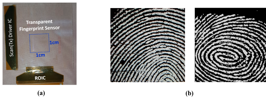
Figure 11. (a) The assembled module of the transparent fingerprint sensing system. ROIC is packaged on COF (chip-on-film) and attached to the panel; (b) measured fingerprint image with pores.
