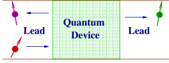
FIG. 1. (Color online) Quantum device with spin-orbit interactions. When a spin-polarized electron with an arbitrary spin orientation is injected from the one lead to the quantum device, it experiences spin-dependent scattering and is transmitted to the other lead. The transmitted and reflected electron spins have a different orientation from the orientation of injected electron spin due to the spin-dependent scattering even though the leads are ideal. This is discussed in detail in Sec. V. In the region of the quantum device, the SO interaction causes the change of the orientation of electron spin in position. In Secs. III and IV, this can be understood in terms of spatial spin precession and nutation, as shown in Figs. 2 and 3. In Sec. VI, both spin precession and nutation are shown to play an important role for spin-polarized transmissions in ballistic semiconductor heterostructures.
