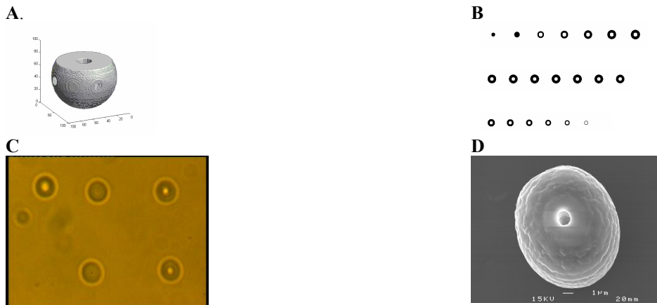
Figure 1 CAD model of the microfabricated sphere (A), 2D bitmaps used to fabricate the micro-object (B), bright field microscope image of 4 \mu\text{m} diameter spheres (C) and SEM image of a 10 \mu\text{m} diameter sphere with 1 \mu\text{m} hollow rod (D).
