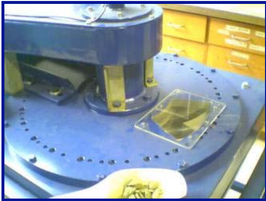
Figure 1: Photograph of the prototype JKRBT device, with rotor-stator showing through the inspection window.
