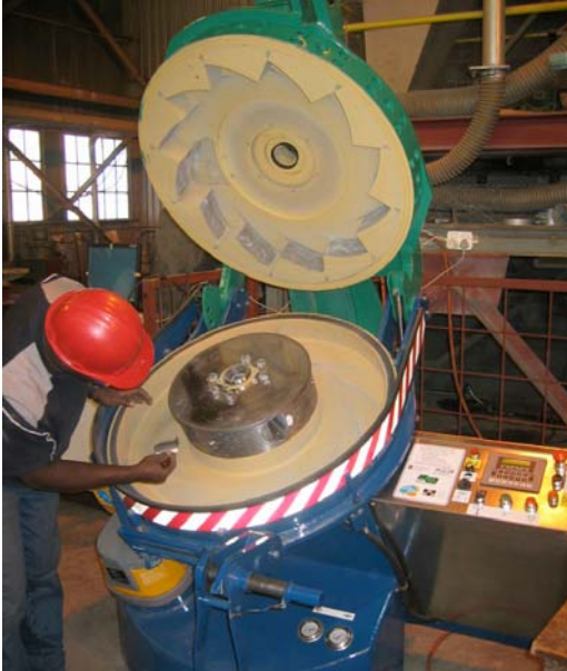
Figure 4: The first industrialised JKRBT installed at Anglo Research in South Africa.
