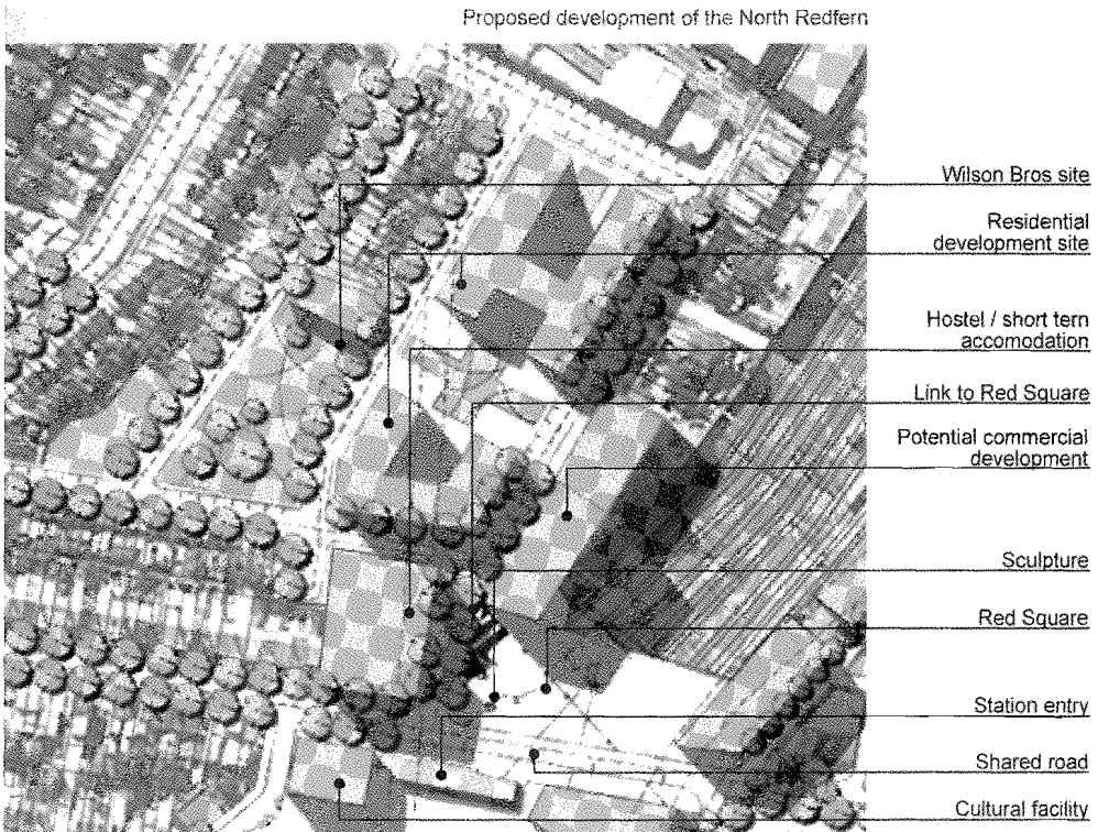
Figure 2 A master plan drawing showing the proposed redevelopment of North Redfern and Red Square prepared by Cox Richardson, Architects & Planners. [Reproduced with the consent of Planning NSW, July 2003.]
