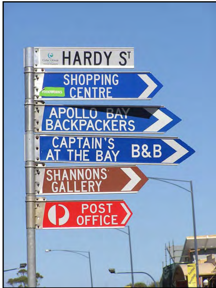
Figure 20: Locating all the signs together can make it difficult to select the one required
