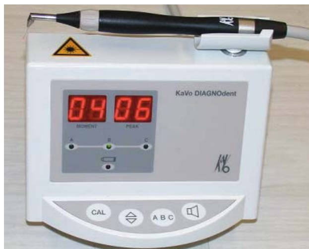
Figure 4. DiagnoDENT "Classic" unit from KaVo, fitted with a prototype sapphire tip for studies of subgingival calculus detection.
