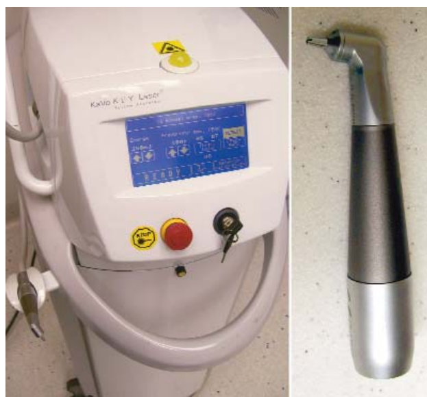
Figure 4. DiagnoDENT "Classic" unit from KaVo, fitted with a prototype sapphire tip for studies of subgingival calculus detection.
