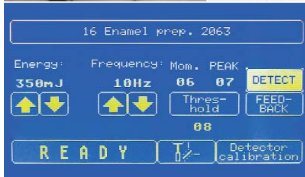
Figure 6. KaVo KEY-3 laser system with autopilot capabilities for removing subgingival calculus and dental caries. The newly released 2063 handpiece (left) and software upgrade (lower panel) allow for specific recognition and ablation of carious dentine.
