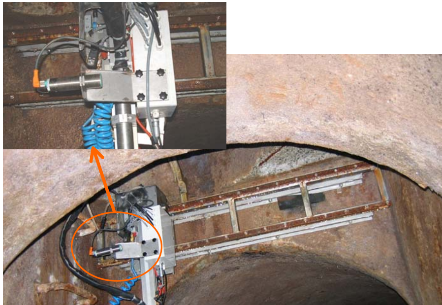
Figure 5 - Two-dimensional sampler Hydre on its rail and detail of the ultrasonic sensor used to control the transverse location
