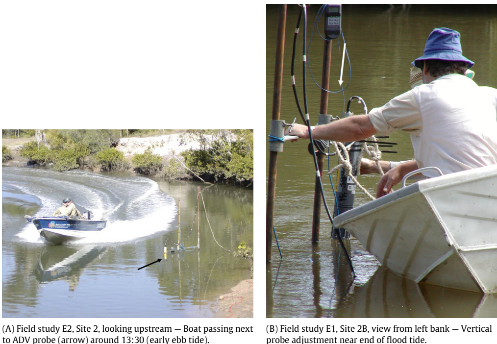
Fig. 3. Acoustic Doppler velocimetry field works in Eprapah Creek estuary.
