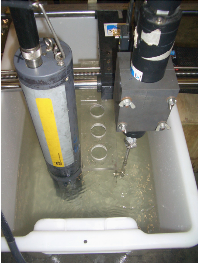
Fig. 2. Photographs of the laboratory experiment 060712b (Eprapah Creek water, sediment sample: 2 (bank material), SSC = 0 g/l (no added sediment)). The YSI 6600 probe is on the left and the microADV system is on the right.
