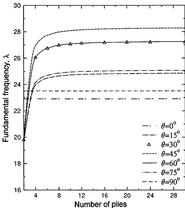
FIG. 4. Effect of number of plies on the fundamental frequency  $\lambda = \omega a^2 \sqrt{\rho/(E_2 h^2)}$  of the laminated S\*S quadrilateral plate ( $\theta/\theta/\theta/\theta/\dots/\theta/\theta$ ) having  $h/a=0.1$ ,  $b/a=0.9$ ,  $c/a=0.7$ ,  $\alpha=65$  deg,  $\beta=75$  deg.
