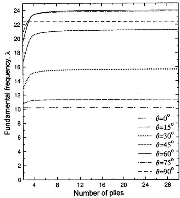
FIG. 5. Effect of number of plies on the fundamental frequency  $\lambda = \omega a^2 \sqrt{\rho/(E_2 h^2)}$  of the laminated CFCF quadrilateral plate ( $\theta/\theta/\theta/\theta/\dots/\theta/\theta$ ) having  $h/a=0.1$ ,  $b/a=0.9$ ,  $c/a=0.7$ ,  $\alpha=65$  deg,  $\beta=75$  deg.
