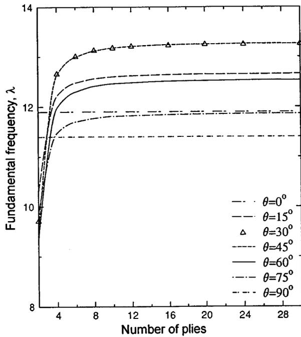
FIG. 3. Effect of number of plies on the fundamental frequency  $\lambda = \omega a^2 \sqrt{\rho/(E_2 h^2)}$  of the laminated CCF quadrilateral plate ( $\theta/\theta/\theta/\theta/\dots/\theta/\theta$ ) having  $h/a=0.1$ ,  $b/a=0.9$ ,  $c/a=0.7$ ,  $\alpha=65$  deg,  $\beta=75$  deg.
