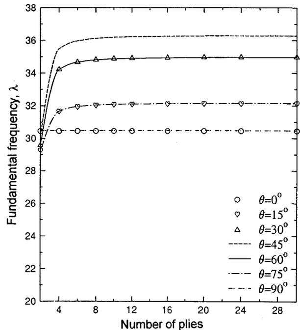
FIG. 2. Effect of number of plies on the fundamental frequency  $\lambda = \omega a^2 \sqrt{\rho/(E_2 h^2)}$  of the laminated CCCC quadrilateral plate ( $\theta/-\theta/\theta/-\theta/...$ ) having  $h/a=0.1$ ,  $b/a=0.9$ ,  $c/a=0.7$ ,  $\alpha=65$  deg,  $\beta=75$  deg.
