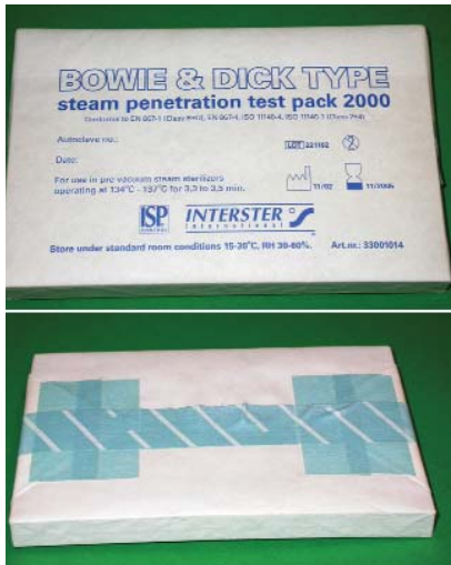
Figure 5. Typical Bowie-Dick test (Interster) used in a pre-vacuum autoclave, which has a "flat pack of cards" configuration.
