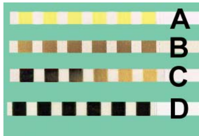
Figure 8. A series of strips from a helix test (unit B from Figure 7), showing an unused strip (A), a series of "fail" results because of incomplete air removal (B-C), and a "pass" result (D) where there has been complete colour change.
