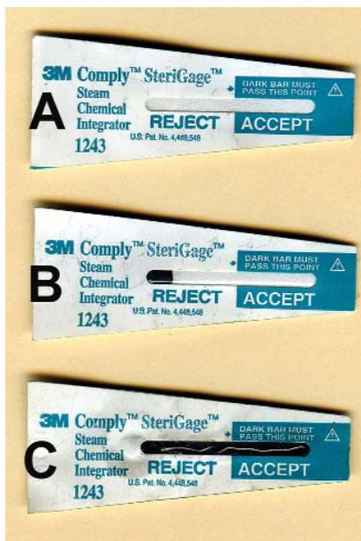
Figure 12. 3M SteriGage™ Class 5 indicators, showing an unused control indicator (A), a “fail” result (B) because of inadequate time (in this case, 2 minutes at 134 degrees), and a “pass” result (C).
