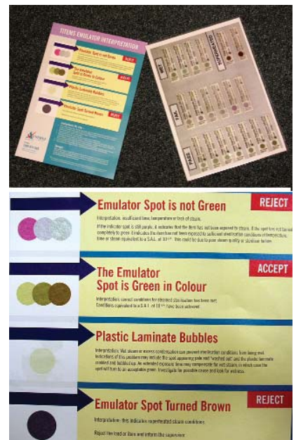
Figure 15. Titems TST™ Class 6 indicators provide a range of useful data on physical parameters, beyond “pass” and “fail” results. For proper interpretation, reference to the manufacturer’s charts is essential.
