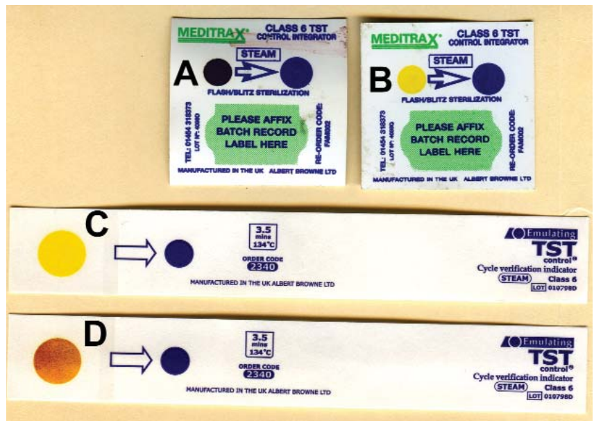
Figure 13. Browne’s Class 6 indicators, which change from yellow to deep purple. The examples shown are a “pass” (A), unused control indicators (B and C), and a “fail” result (D) with partial colour change (60 seconds/134 degrees).
