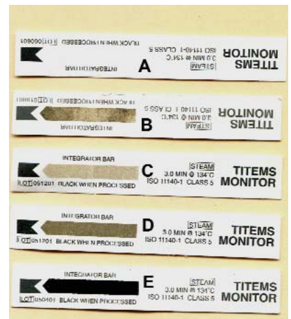
Figure 11. A series of Titem's Class 5 chemical indicators. The topmost indicator (A) is unused, and the subsequent indicators show the colour change at 90 seconds/134 degrees (B), 2 minutes/132 degrees (C), 2 minutes/134 degrees (D), and 3 minutes/134 degrees (E). Note how the colour intensity is less when the temperature is too low (compare C with D).
