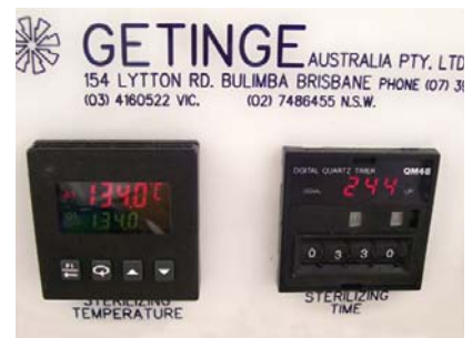
Figure 4. Autoclave with user-adjustable time and temperature parameters, used for research and teaching into sterilization technology.
