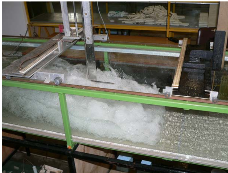
Fig. 2 - Air entrainment in hydraulic jump - Fr_1 = 8.3 , x_1 = 0.75 m, d_1 = 0.018 m, shutter speed: 1/80 s, flow from right to left
