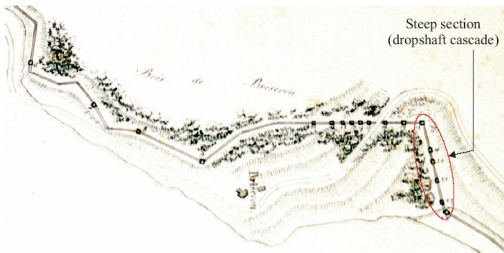
Fig. 7 - 19th century drawing of the Montjeu aqueduct steep section at Brisecou, Planche 65, Roidot-Del age (1879?)
