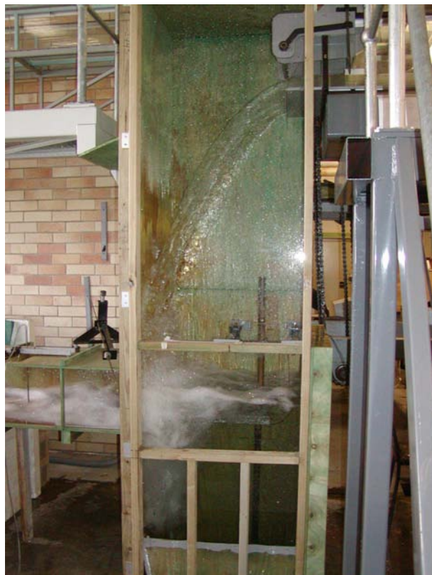
Fig. 6 - Full-scale hydraulic model of the Recret dropshaft, Yzeron aqueduct (Lyon, Fra) - Model flow rate: Q = 0.044 \text{ m}^3/\text{s}
