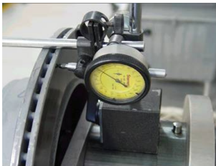
Figure 1 Measurement of lateral run-out
