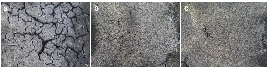
Figure 4. Photographs of combustion residues for a 10; b 20; and c 30 wt% organoclay in polyamide 6 matrix.
