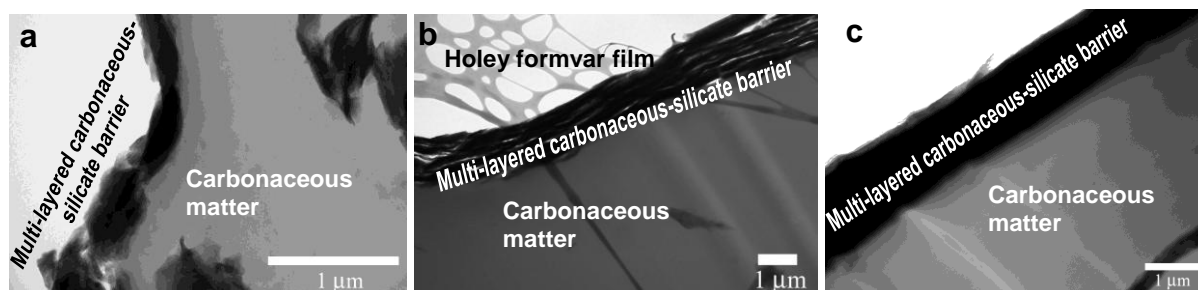
Figure 5. Low magnification TEM micrographs of cross-sections beneath the top surfaces of combustion residues of polyamide 6 nanocomposites with a 10; b 20; and c 30 wt% organoclay.
