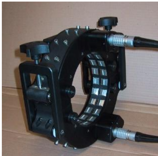
FIGURE 3. Solid transducer assembly for 8 inch pipe showing array of dry coupled piezoelectric transducers.
