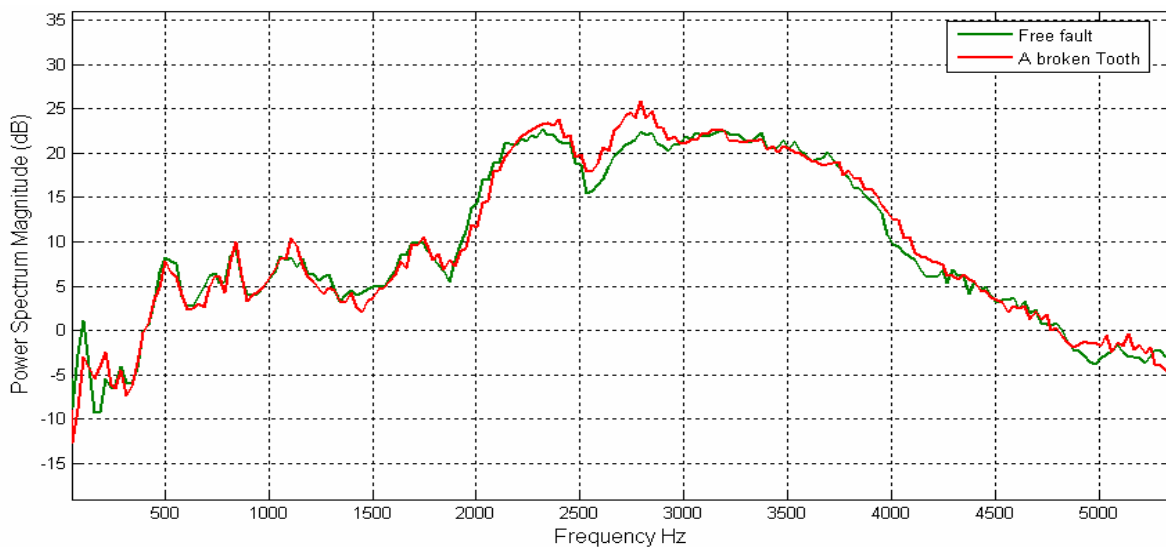
Figure 5 PSD of the averaged signal for different sensors, for the fault-free case and a broken tooth
