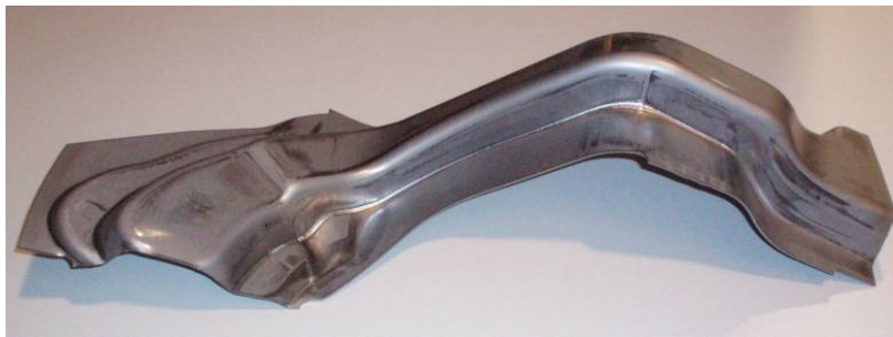
Figure 2 Reinforced rear suspension support
