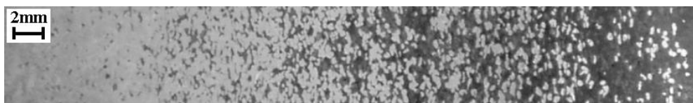
Figure 1. Picture of the Al-PC FGM where light areas are aluminium while dark areas are polycarbonate.
