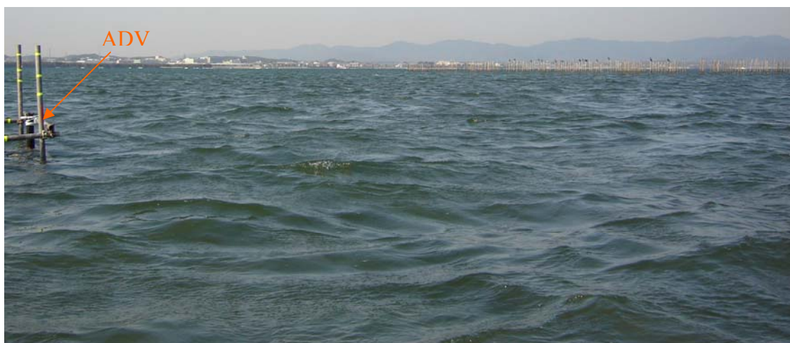
Figure 9.4 – Photograph of wind waves observed at Site 1 Hamana Lake taken during installation for study HLJ1 on 24/11/05, with poles holding ADV on far left.
