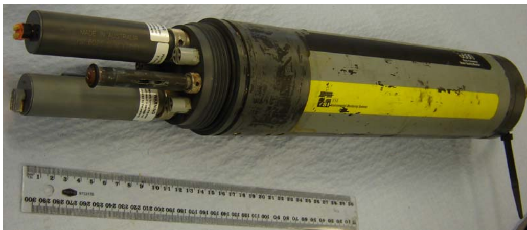
Figure 3.10 – YSI6600 probe with sensors exposed.
