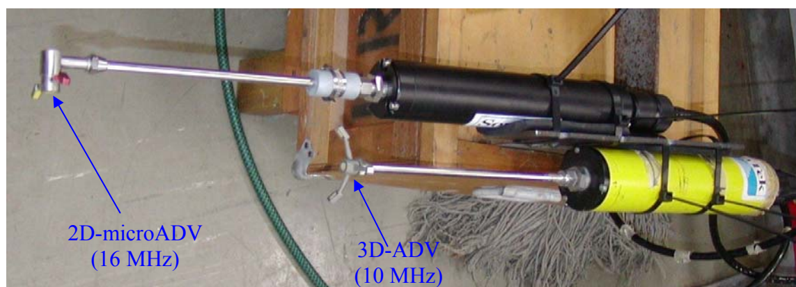
(B) Configuration of 3D-ADV and 2D-microADV used during field studies E6 and E7. Photograph by H. Chanson during preparation for study E6 (16-18/05/05).
