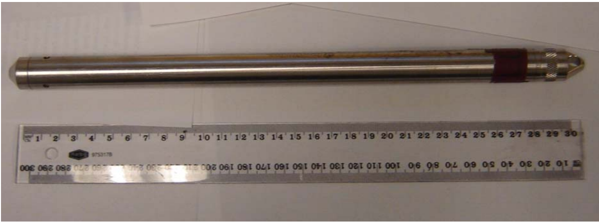
Figure 3.13 – In-Situ mini-Troll probe.
