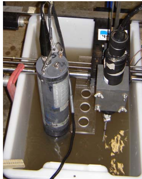
(B) Test tank with 28.35 g of sediment added (SSC = 0.71 g/L).
