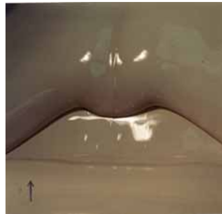
Figure 2: "Laminar" hydraulic jump in the free surface flow of a mud in an inclined channel (width=20cm). The flow direction is indicated by the small arrow. The fluid from upwards (supercritical) has a large velocity and small thickness, it penetrates the fluid downwards flowing with a larger thickness in the subcritical regime.
