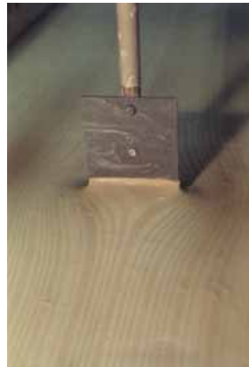
Figure 3: Channelized flow of a mud: flow around an obstacle, parallel lines have been drawn upstream on the free surface, these lines deform as the fluid passes over the obstacle.
