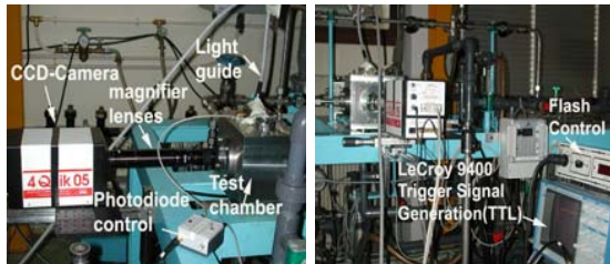
Figure 4. The apparatus of the visualization system.
