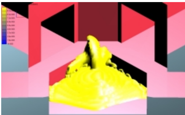
Fig. 13 Dust iso-contours or iso-surface ( 100\text{mg}/\text{m}^3 ) (full bin scenario) (A snap shot of transient/time dependent case)
