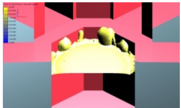
Fig. 10 Dust iso-contours or iso-surface ( 100\text{mg}/\text{m}^3 ) (empty bin scenario) (A snap shot of transient/time dependent case)
