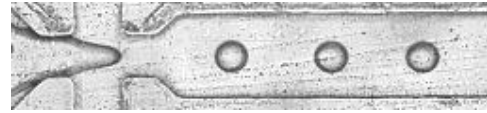
Figure 2: A picture of the microfluidic chip with water-in-oil droplets formed. The width of the channel at the cross was 105\mu\text{m} and the depth is 70\mu\text{m} .
