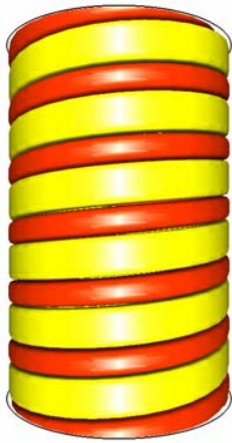
Fig.4. Laminar spirals in the system of infinite counter-rotating cylinders. Ri=110 , Ro=0 , \eta=0.8 .
