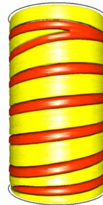
Fig.3. Laminar spirals in the system of concentric cylinders with endplates. Re=300 , \eta=0.75 , \Gamma=12.98 , f_s / f_r = 0.35 . Isosurfaces show +/- radial velocity
