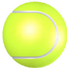
Figure 4: 3D CAD Model of tennis ball with Sim (2 mm w)
