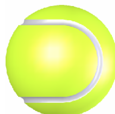
Figure 5: 3D CAD Model of tennis ball with bigger seam dimension (5 mm w)
