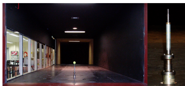
Figure 1: A front view of experimental set up in RMIT Industrial Wind tunnel with a motorised supporting device (right)
