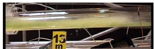
Figure 4. Time traces of liquid fraction probes (no. 1 at the top) and of pressure in bar (at the bottom). 1 degree upwards pipe inclination, U_{sg} = 4.34 m/s and U_{sl} = 0.13 m/s. The video snap shot is for the wave enclosed in the first rectangle (green).
