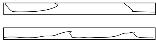
Figure 1. Sketch of a slug (top) and large amplitude waves (bottom)
