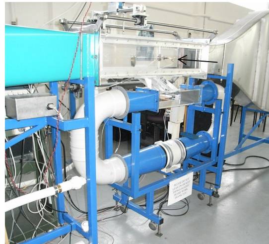
Figure 6. Completed supply loop installed. Flow from right to left.
