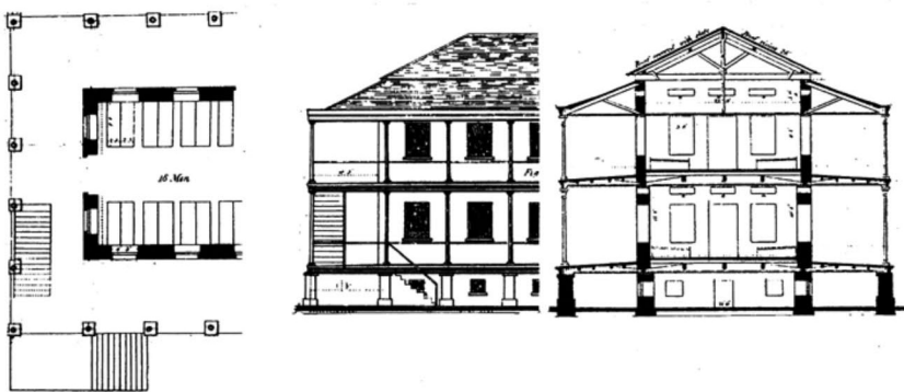
Final version of Uniform Barrack System as erected at: Barbados, (single storey hospital and iron barrack), Bahamas, Antigua, St. Vincent, St. Lucia and Grenada.
