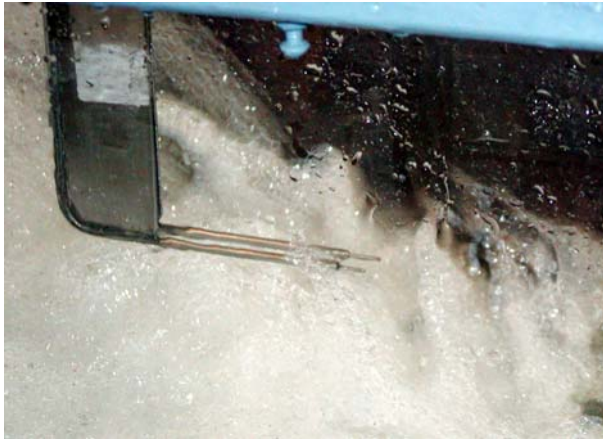
Fig. 3 Photograph of two single-tip conductivity probes side-by-side in a hydraulic jump ( Fr_1 = 7.9 , \rho_w \times V_1 \times d_1/\mu_w = 9.4 \text{ E}+4 )—Flow from right to left
