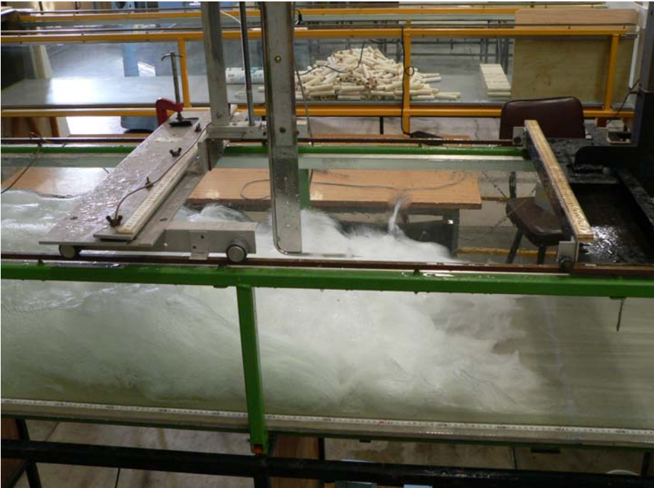
(D) Flow conditions: Fr = 8.3 , x_1 = 0.75 m, d_1 = 0.018 m, shutter speed: 1/20 s, flow from right to left
