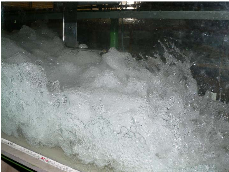
(C) Jump toe and roller - Flow conditions: Fr = 8.3 , x_1 = 0.75\text{m} , d_1 = 0.018\text{m} , shutter speed: 1/250 s, flow from right to left
