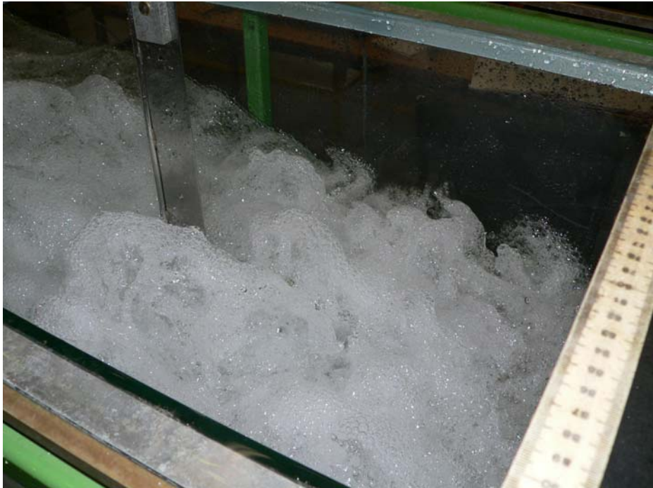
(C) Jump toe and roller - Flow conditions: Fr = 8.3 , x_1 = 0.75\text{m} , d_1 = 0.018\text{m} , shutter speed: 1/250 s, flow from right to left
