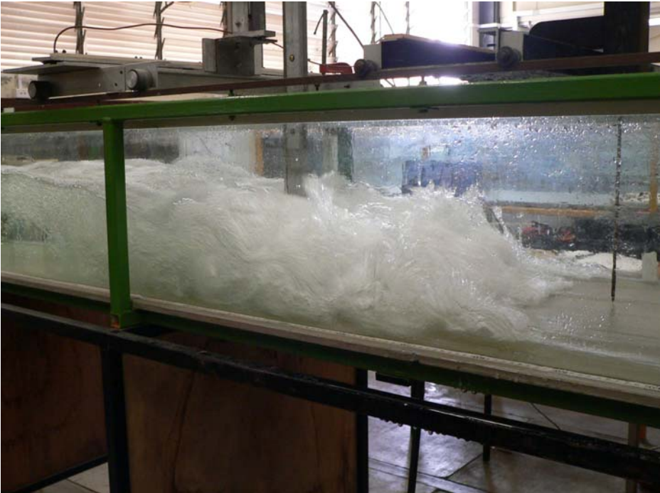
(D) Flow conditions: Fr = 8.3 , x_1 = 0.75 m, d_1 = 0.018 m, shutter speed: 1/20 s, flow from right to left
