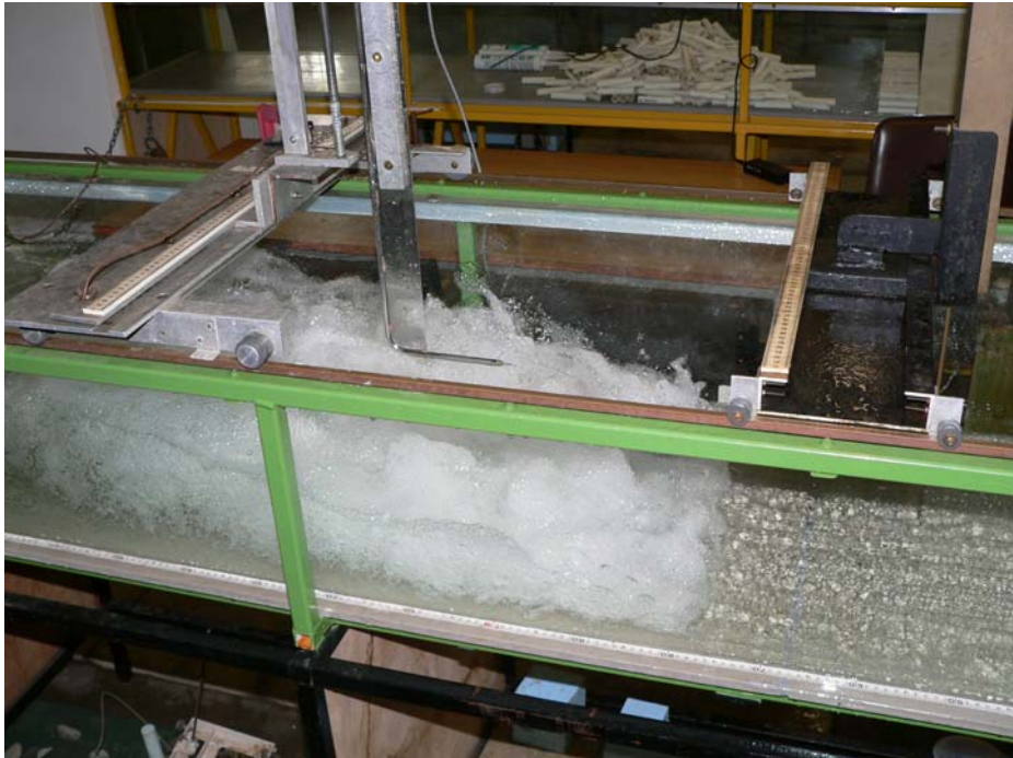
Fig. A.3 - Details of the air-water flow structures above the hydraulic jump
