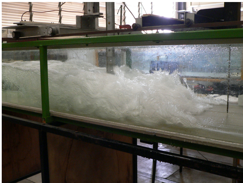
General view of the hydraulic jump (Flow from right to left): Fr = 7.6 , x_1 = 0.75 m, d_1 = 0.018 m
