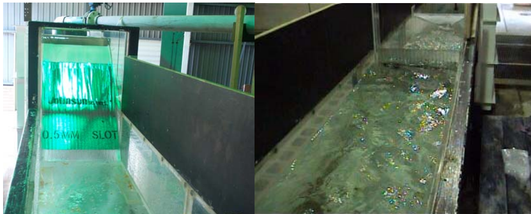
Figure 4. General view of the flume showing the Coanda screen (left) and the vertical plate screen (right).
