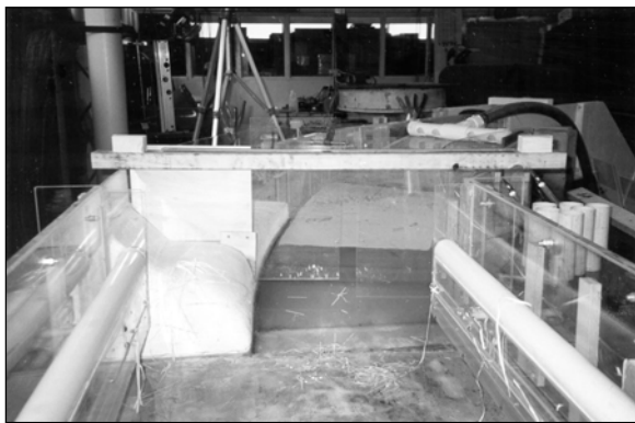
Figure 8 – Side-Crest Weir and Pond Baffle Plate
