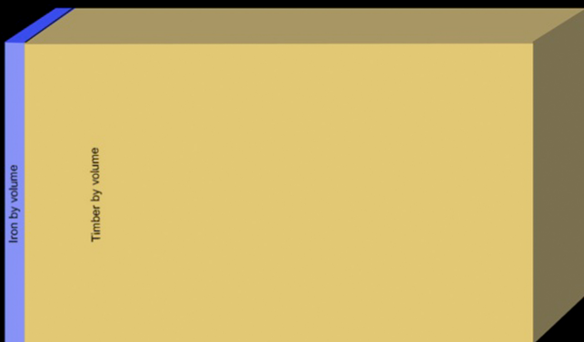
Comparison of volumes of Iron and Timber used in the Crystal Palace
