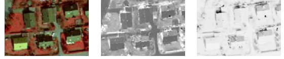
Figure 6: CIR image (left), NDVI (centre) and \sigma_{NDVI} (right). In the \sigma_{NDVI} image, white areas correspond to low \sigma_{NDVI} .
