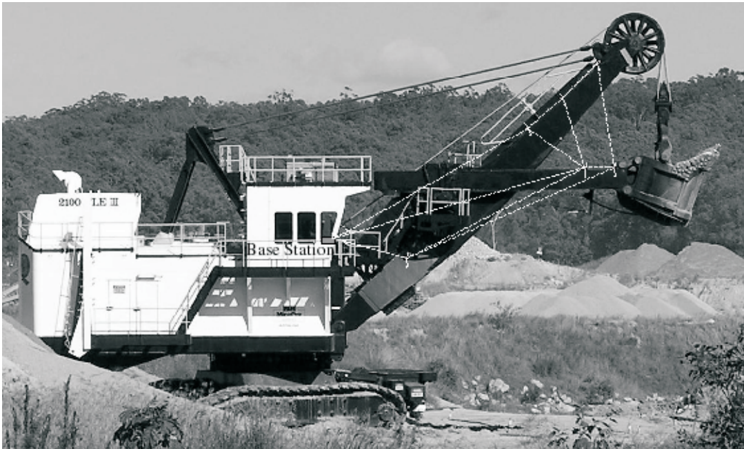
FIG 3 - Layout of trial sensor network on the 2100 BLE P&H/CRCMining electric rope shovel. The base station will be located inside the operators cabin and sensor nodes distributed around the handle and boom. Note that sensors on the non-visible side of the shovel will also be used, with a transfer node located on the shovel house body for transmission to the base station.
