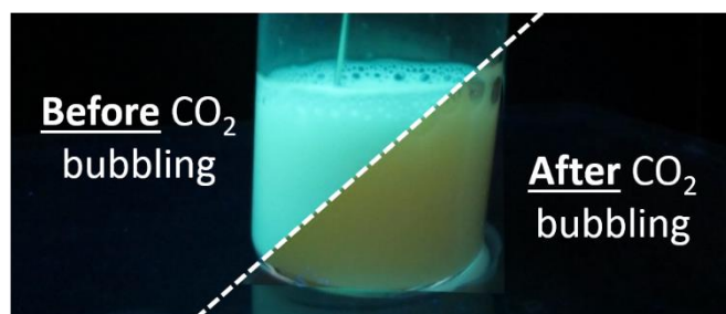
Figure 4.16. Pictures of particles ( FRP-360 ) before and after \text{CO}_2 bubbling observed under a UV lamp at 345 \text{ nm} .
