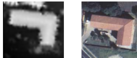
Figure 3. Left: DSM of a building (grid width: 0.5 m). Right: aerial image (ground resolution: 0.17 m). Length of the larger wing of the building: 30 m.
