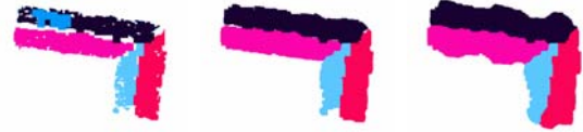
Figure 5. Left: planar segments after region growing. Centre: the segments after morphologic filtering and merging of co-planar segments. Right: Voronoi diagram.
