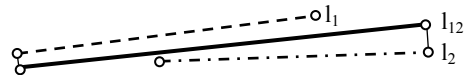
Figure 6. Matching and merging edge segments. l_1 and l_2 : edges from images 1 and 2. l_{12} : combined edge, covering the projections of both l_1 and l_2 .
